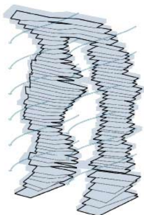
Double slabs house \text{CO}_2 chambers and allow for cross-ventilation that cools the units above and below
